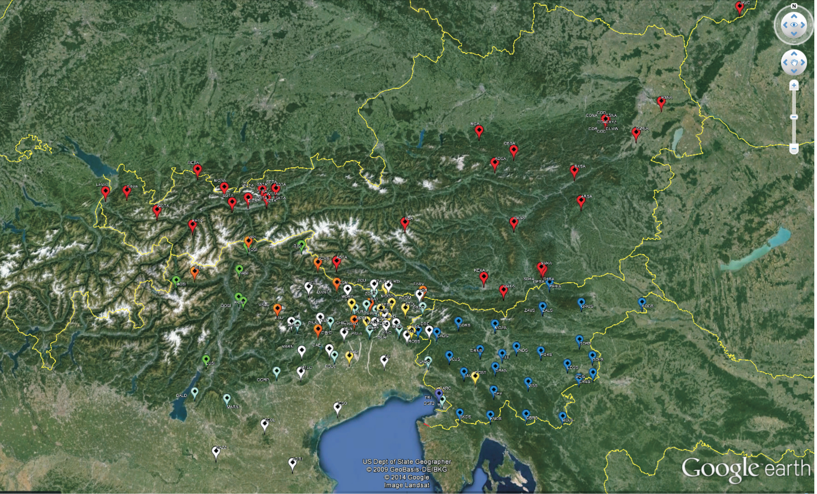
Map of the Southern Alps area with the CE3RN stations, red symbols: Austrian national BB network (ZAMG - OE); white symbols: Friuli Veneto SP network (OGS - FVG); yellow symbols: Friuli VG accelerometric network (DMG - RF); light blue symbols: NE Italy BB Network, (OGS & DMG - NI); blue symbols: Iovene national BB network (ARSO SL); green symbols: South Tyrol BB Network, (BOLZANO - SI).
